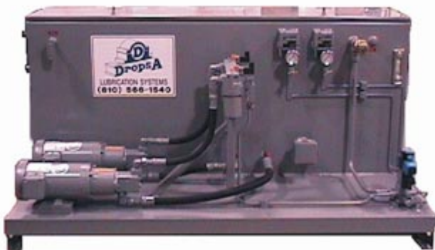
Large Oil Pump Package Supplied on Recent Air/Oil Installation
